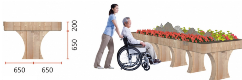
Figure 3. Elevations and Renderings of the "horticultural therapy planting box" (length unit: mm)
