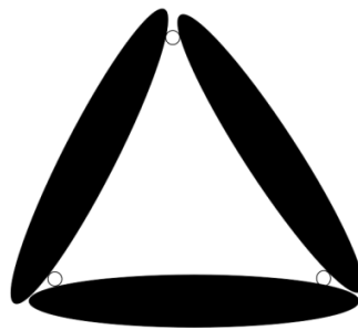
Figure 2. Articulated triangle with three rigid body
