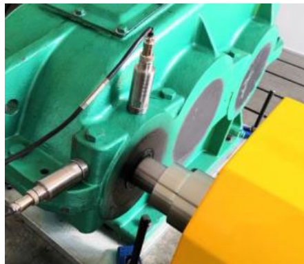
Figure 5. Field vibration data acquisition measurement point arrangement
