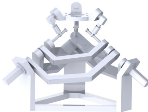
Figure 1. 3-RRCP parallel pointing mechanism model
