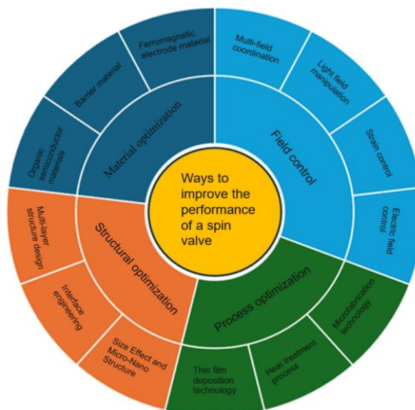
Figure 2. Classification of spin valve performance improvement methods
