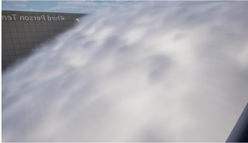
Figure 2. Volumetric fog material with distance-field gradient and soft boundary attenuation (Photo credit: Original)
