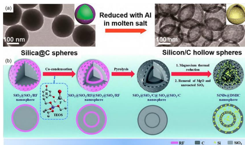
Figure 2. A visual representation of common silicon-derived hollow sphere/cage anode materials. (a) the creation procedure of cavitated, porous silicon spheres utilizing a molten salt reduction technique [2]. (b) The accompanying diagram depicts the creation of SiNDs@DSHC nanospheres, following the methodology [3].
