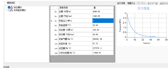
Fig 1. Natural gas pipeline venting software operating interface
