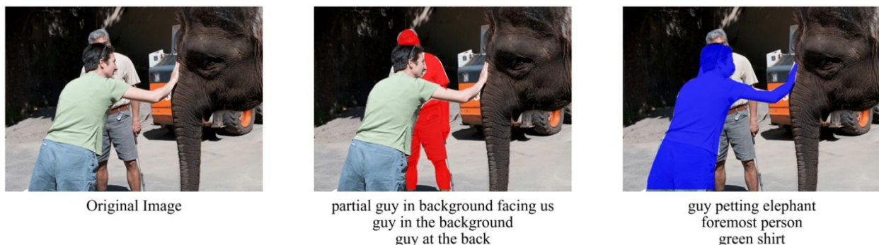
Fig. 1 The task of RIS is to predict a mask of the instance based on image and referring expression. Each instance could be referred by a few different expressions.
