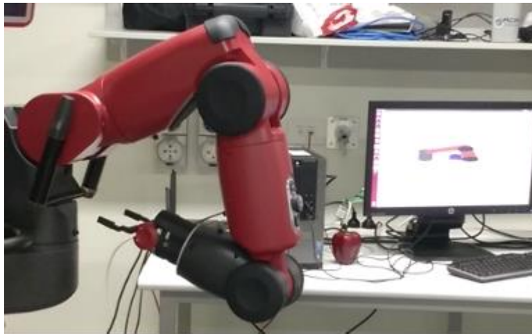
Fig. 1 Baxter's arm being controlled by a trained deep Q Network (DQN). Synthetic images (on the right) are fed into the DQN to overcome some of the real-world issues encountered, i.e., the differences between training and testing settings [1].
