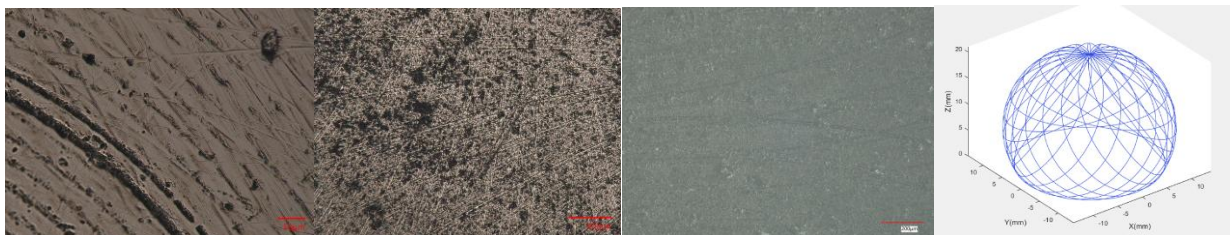
Figure 16. The trajectory morphology obtained by polishing and its simulation results
