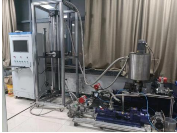
Fig.1 Visualization device for dynamic migration of pulverized coal in coalbed methane wells
