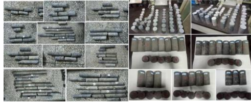
Figure 1. Underground Borehole Coring, Sampling and Rock Sample Preparation
