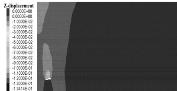
Figure 2. Displacement field at 20m advance
