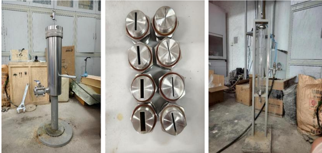
Fig. 2 Lost-circulation simulation experimental apparatus
