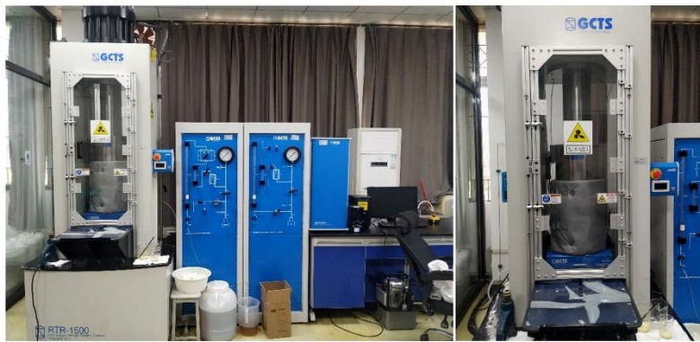
Fig. 4 High-temperature and high-pressure integrated rock testing system
