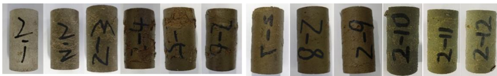
Fig. 9 Morphology of cement specimens after conventional triaxial compression tests
