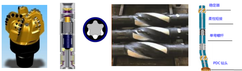
Figure 1. Integrated “four-in-one” BHA
