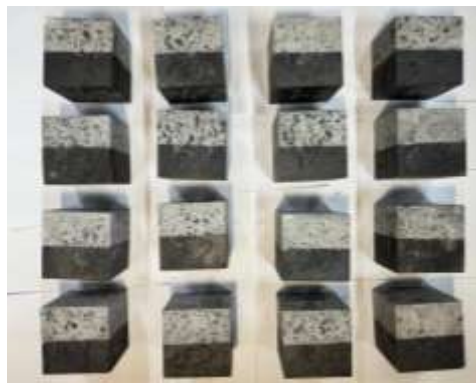
Figure 2-2 Finished products of samples with different gangue gradation
