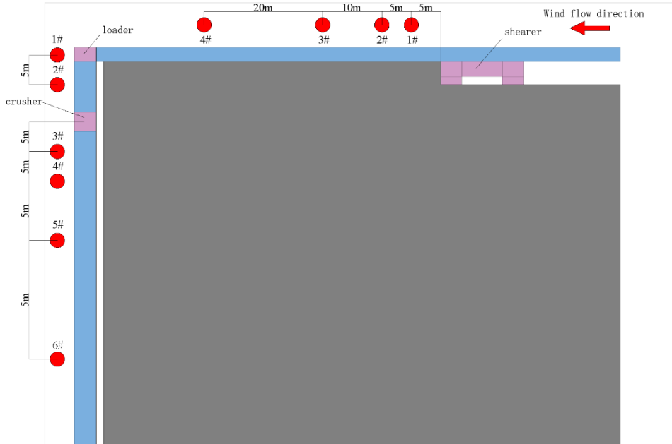
Fig. 2: Schematic Diagram of Dust Monitoring Points in the 5011 Mining Face
