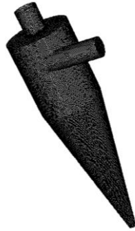
Fig. 1 Mesh model of 250 mm diameter cyclone
