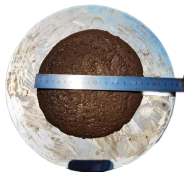
Figure 2-1. Schematic of fluidity test
