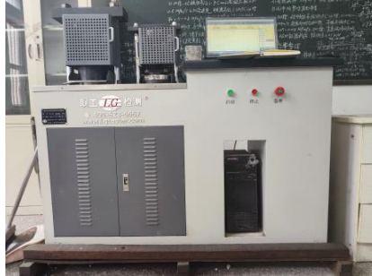
Figure 2-2. Flexural and compressive testing machine
