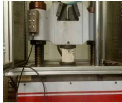
Figure 6. Test block pressurization
