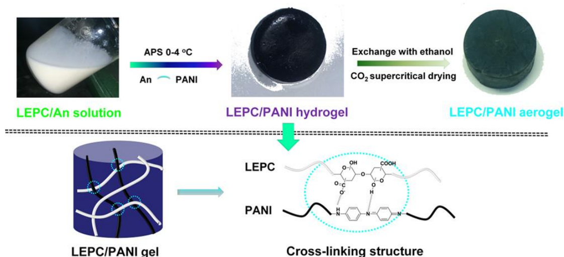
Figure 10. Schematic illustration of LEPC/PANI aerogel formation and its cross-linking structure[24]
