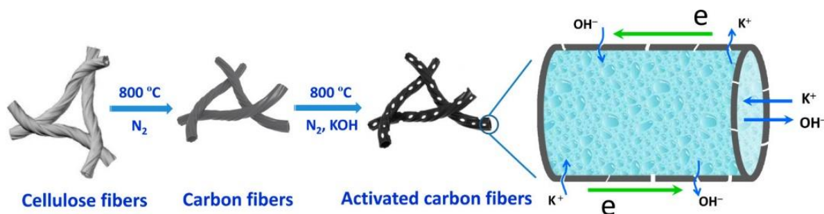
Figure 6. Schematic Illustrating the Fabrication Steps and Ion/Electron Transport Behavior in aCF Electrode [17]
