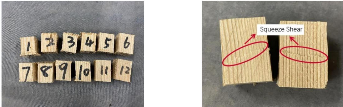
Figure1. Failure mode of compression specimen along grain
