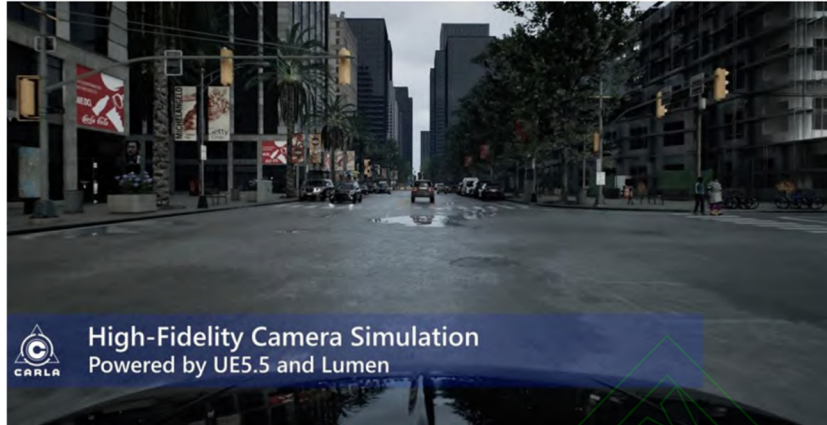
Figure 5. Driving scenario in the CARLA simulator, leveraging Unreal Engine rendering capabilities to generate realistic simulated environments via sensors
