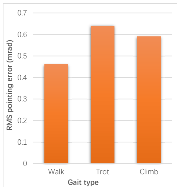
Figure 4. RMS pointing error during walk, trot and climb gaits showing stable sub milliradian accuracy under locomotion.
