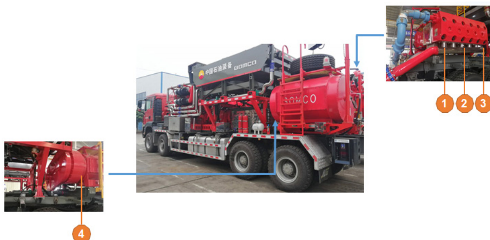
Fig 7. Vibration measurement point installation location
