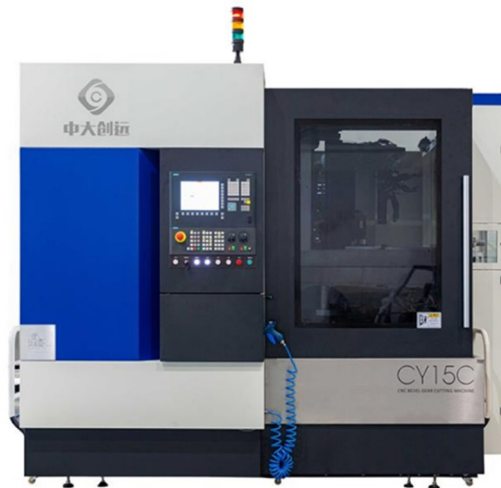
Figure 3. CY15C spiral bevel gear milling machine
