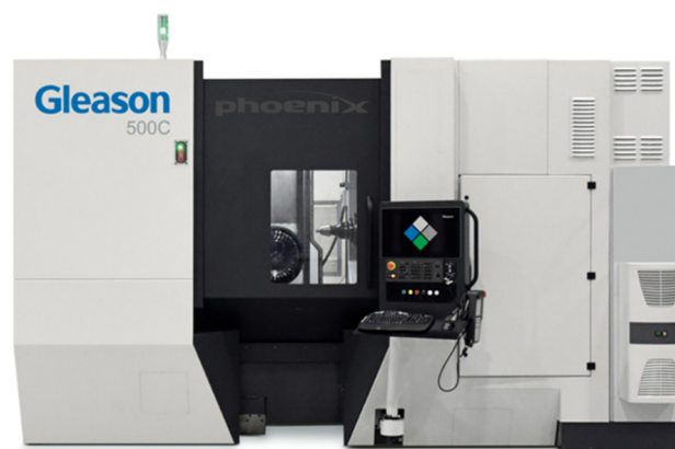
Figure 1. Gleason Phoenix series bevel gear milling machine
