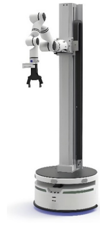
Figure 1. Model of the Adjustable-Height Single-Arm Mobile Manipulator
