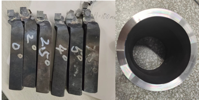
Fig 12. Experimental casing with cutting tooth
