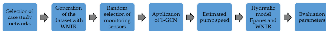
Figure 2. Workflow for developing a digital twin for water distribution networks, adapted (Bonilla et al., 2022).
