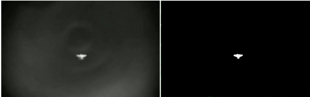
Figure 2. Otsu's Binarization Effect on a Sky Background
