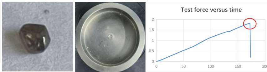
Fig 11. Medium-grade diamond. Particle Size: 2.0mm, Peak Test Force: 1.82kN
