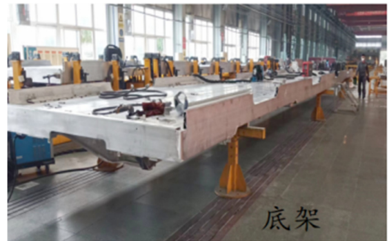
9-d: The device is placed on the ground to support the side wall welding parts 9-e: The device is placed on the I-beam to support the bottom frame welding parts
