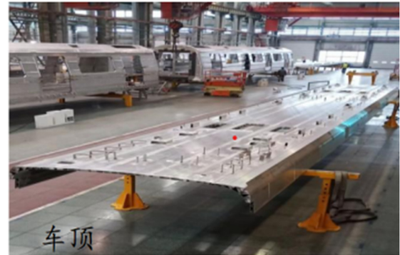
9-b: The device is placed on the I-beam and fixed to support the reverse welding parts on the roof 9-c: The device is placed on the ground to support the normal welding parts on the roof
