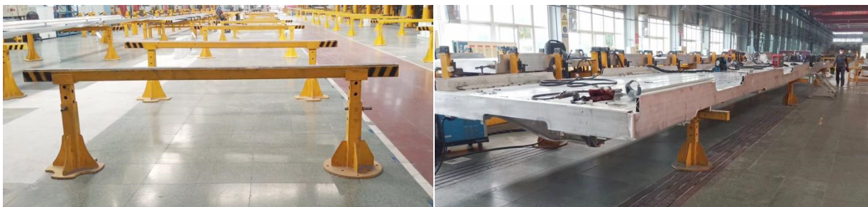
Figure 12. Tool verification was carried out in the production of Harbin Metro underframe to meet technical requirements
