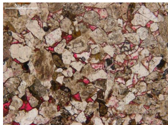
(b) Intragranular corrosion pore
