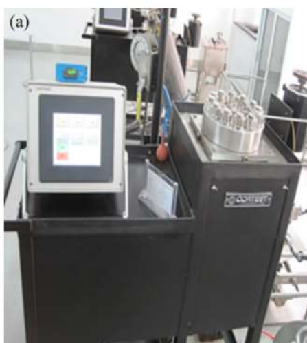
Figure 2. High-temperature and high-pressure dynamic reactor experimental device
