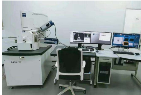
Figure 1. ZEISS SIGMA 300 field emission scanning electron microscope
