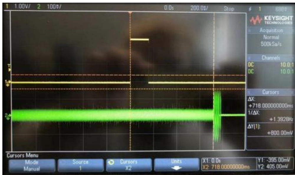
Figure 20. vertical cursors in orange shows the audio latency (signal on top shows when button has been pressed, signal on bottom shows when the audio signal comes out)
