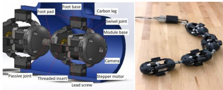
Figure 11. Multi-module peristaltic robot
