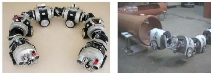
Figure 12. Multi-joint worm-like pipeline robot
