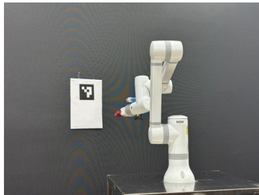
Figure 4. Hand-eye calibration process
