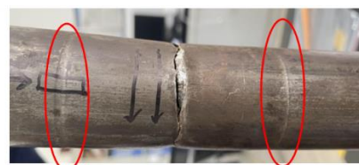
The lateral trauma to the tube caused by the clamping block stack is the same, such mechanical trauma will reduce the plastic toughness of the tube, so that the tube has the risk of fracture.
