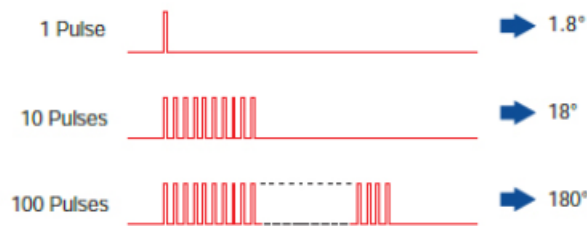
Figure 3. Proportional relationship between rotation distance and pulse number
