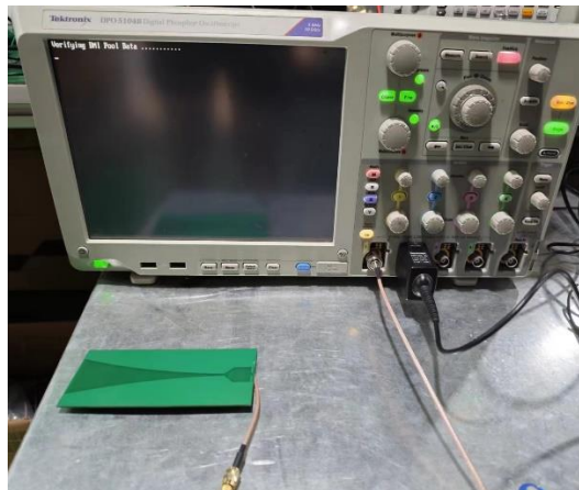
Figure 3.1. Construction of partial discharge waveform acquisition environment
