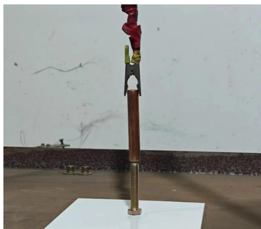
Figure 2.8. Internal discharge model
