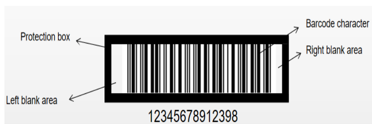
Figure 4-1. The ITF-14 symbol structure
