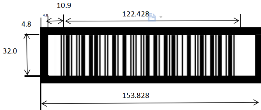
Figure 4-4. ITF-14 barcode dimensions
