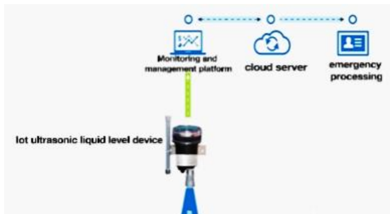
Figure 1-2. Detection of sensing through ultrasonic sensors combined with IoT [6]
