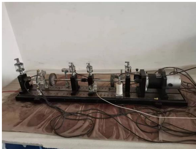
Figure 4: Sliding bearing rotor test rig
